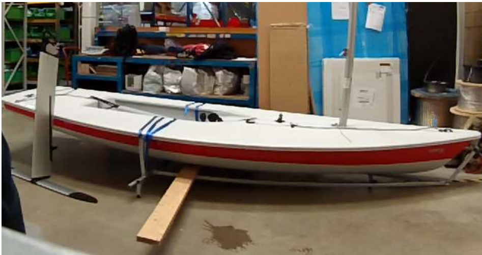
Method to support the centrecase insert from below when fitting the gear block.
