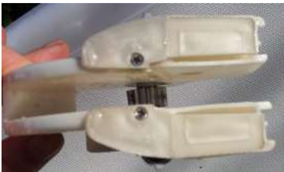
Fig 15 Gear block with packers attached with screw
