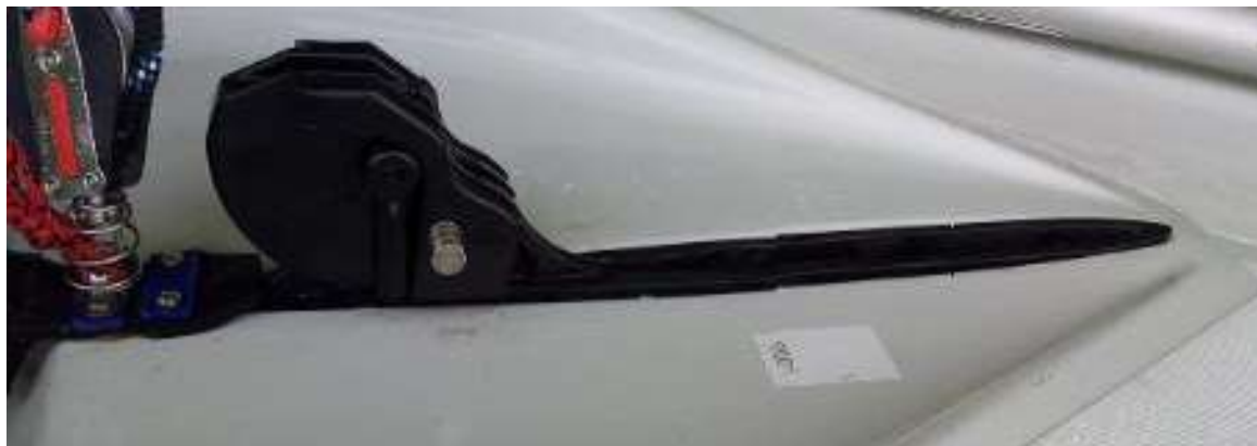
Gear block with retaining pin inserted through the centrecase insert from the starboard side
