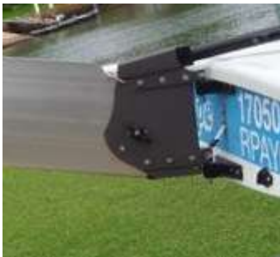
Fig 19 Showing the rudder blade in the retracted position and fully deployed
