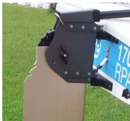
Fig 19 Showing the rudder blade in the retracted position and fully deployed
