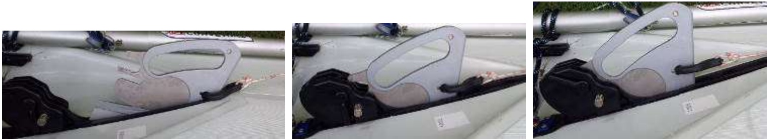
Fig 15 Pull board down and aft to engage in gearblock. Pull the board down until the clip sits on the deck, then pull the board backwards to engage the gear block.
