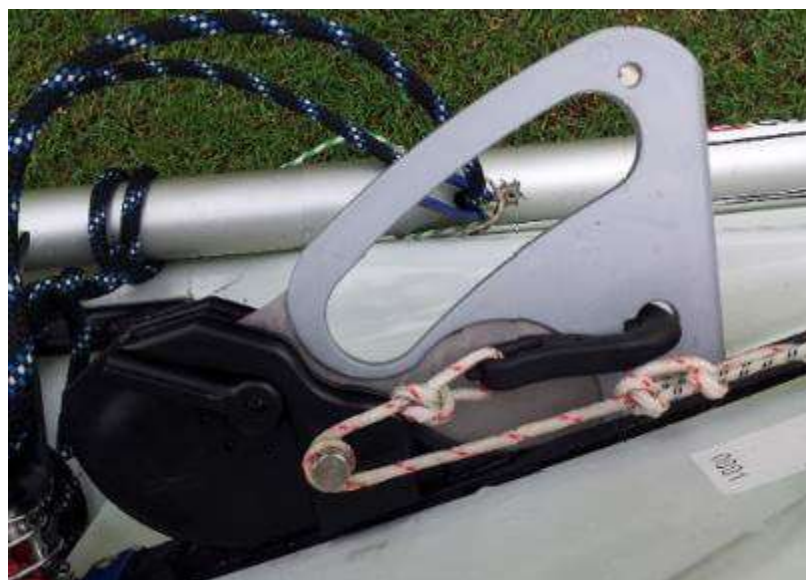
Fig 15 Once engaged in the gear block, rotate the large retaining clip 180 degrees and wrap the cord around the pin with one complete turn as shown.
