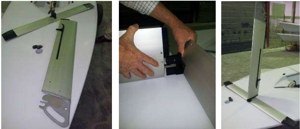
Fig 11 Assembly of Centreboard foil GF001 and lifting foil GF002
