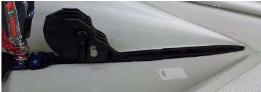
Fig 10 Gear block with retaining pin inserted through the centrecase insert. GF007
