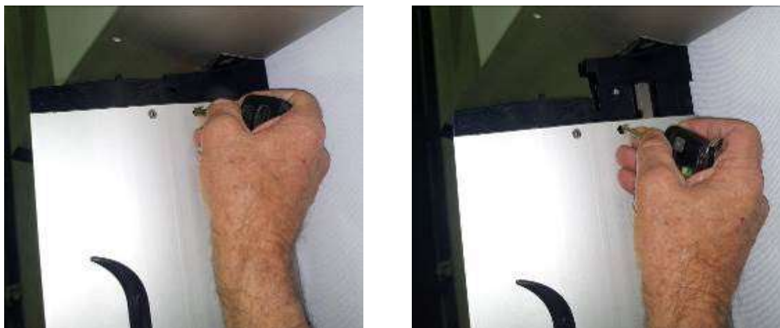
Fig 12 Depress the spring clip and pull the foils apart.
