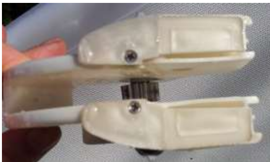
Fig 11 Gear block with packers attached with screw
