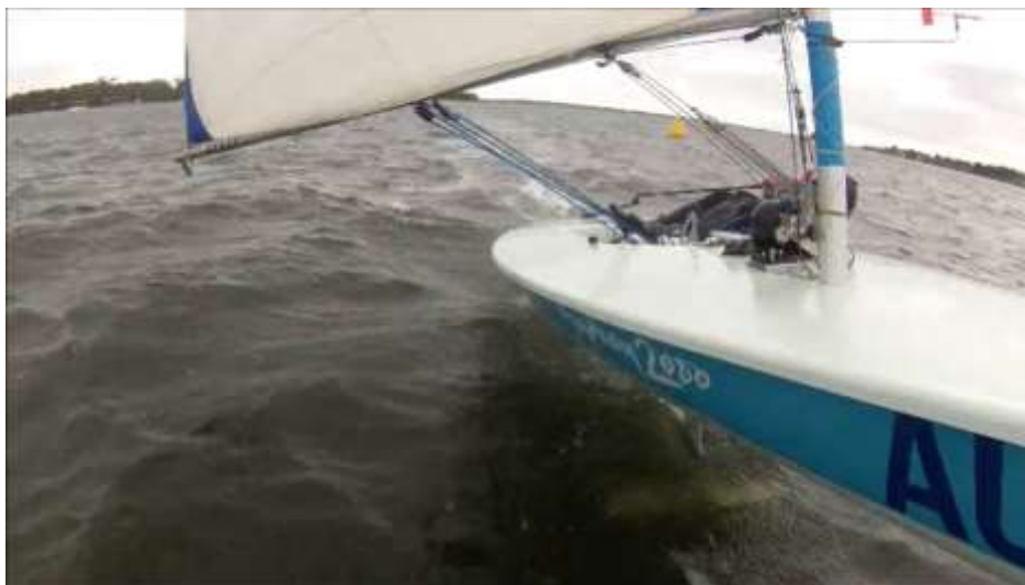
Foiling at speed: Note centre boom sheeting for responsive trimming.
